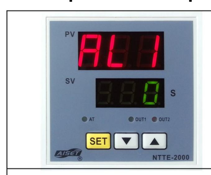
press **SET** button 4 seconds to enter into interface as picture.
