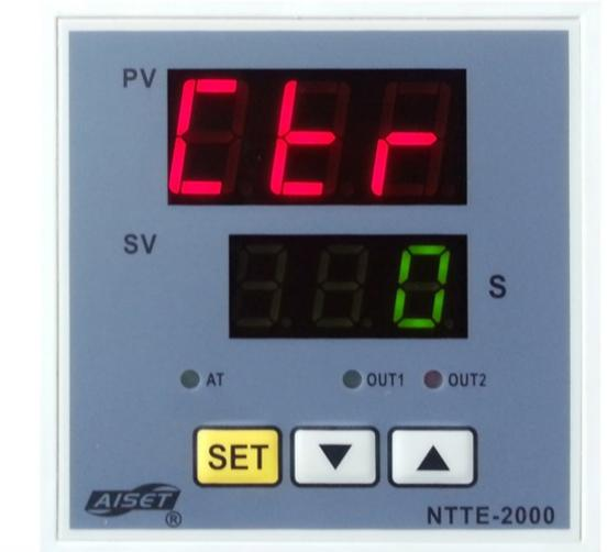
Press SET button to enter into next interface, then press SET to choose the "ctr" interface as picture, press "△" and "▽" to change "SV" no as 0(for Celsius) or 1(for Fahrenheit). press SET 4 seconds to quit.
