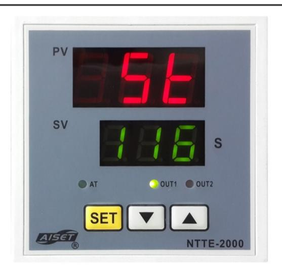
Press SET button second time, the PV part shows "st". Press arrows "△" or "▽" to set time.
