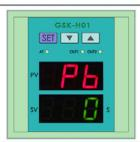
press SET to choose "pb" interface as picture,then Press "△" and "▽" to set temperature compensation numbers. For example,if the real temperature is 15 °C higher than control board shows,pls input +15 into the AV part,if the real temperature is 15°C lower than control board shows,pls input -15 into the AV part. press SET 4 seconds to quit.
