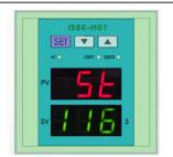
Press SET button second time, the PV part shows "st". Press arrows "△" or "▽" to set time.
