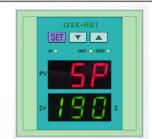
Press still button first time, the PV part shows "sp". Press arrows " $\triangle$ " or " $\nabla$ " to set temperature.
