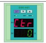
Press SET button to enter into next interface, then press SET to choose the "ctr" interface as picture, press "△" and "▽" to change "SV" no as 0(for Celsius) or 1(for Fahrenheit). press SET 4 seconds to quit.
