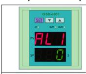
press **SET** button 4 seconds to enter into interface as picture.
