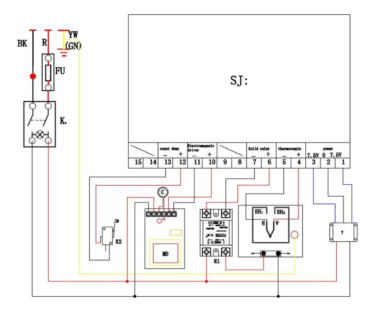
K<sub>0</sub>: Power Switch T: Transformer EH1 EH2: Heating Pipe C:Magnet FU:Fuse MD: Magnet Driver K2: Limit Switch R1: Relay SJ: Digital Controller
