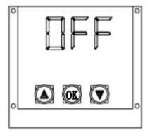
2. Press the "OK" button will show the degrees Celsius "C". You could use the Up or Down button to switch between degrees Celsius and degrees Fahrenheit.
