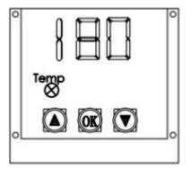
4. Press "OK" button to enter TIME setting. When the TIME indicator blinks, use Up/Down button to set the required time. (Time adjustable range: 0-999S)
