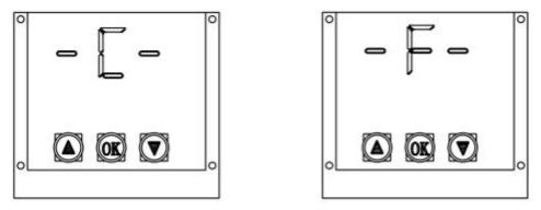
3. Press "OK" button to enter TEMPERATURE setting. When the TEMP indicator blinks, use Up/Down button to set the required temperature. (Temperature adjustable range: 100-225 C/212-437 F)
