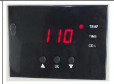
Press button, the temp light is on. Select with arrows the temperature according to different transfer material (Normally 180° ~200°)
