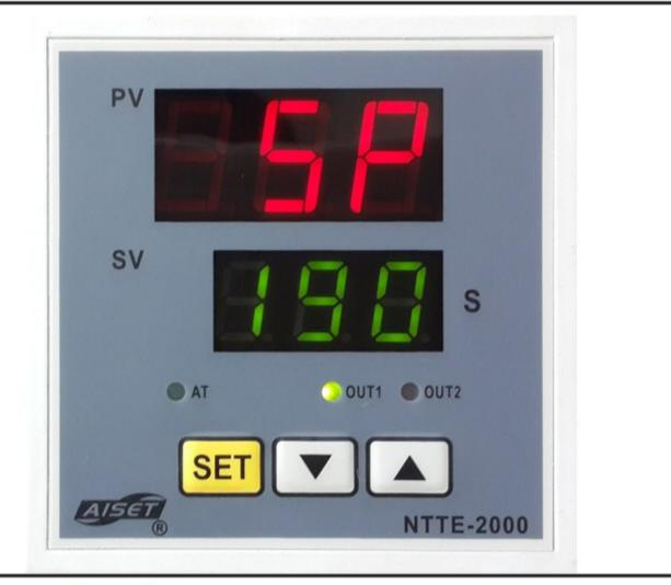
Press  $\P$  button first time, the PV part shows "sp". Press arrows " $\triangle$ " or " $\nabla$ " to set temperature.
