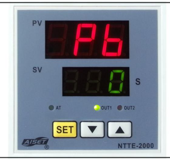
press set to choose "pb" interface as picture, then Press "△" and "▽" to set temperature compensation numbers. For example, if the real temperature is 15 °C higher than control board shows, pls input +15 into the AV part, if the real temperature is 15 °C lower than control board shows, pls input -15 into the AV part. press set 4 seconds to quit.
