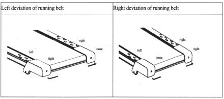
Note: Running belt deviation is not covered by warranty, and is mainly maintained and maintained by users according to the instructions
