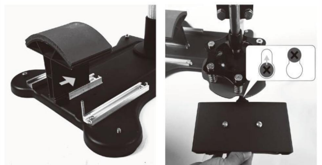
Place the hat element on the bottom bracket. Push it to the end
