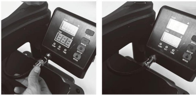
Insert the cable into the aviation plug
